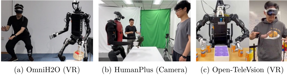
Figure 3.1: Recent data collection methods utilizing shadowing. In all three works humanoid robots are mimicing human actions using vision-based motion retargeting.
