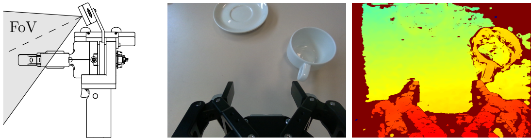
Figure 4.3: Left: observation camera field of view (FoV). Right: example RGB and depth image observations.
